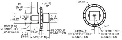
The unique electric switch design in the Series 1640 Floating Contact Null Switch for High and Low Actuation is another Dwyer Instrument, LLC innovation. The Dwyer Model 1640 Differential Pressure Switch resembles the high precision large diaphragm Series 1630 switches. However, the Model 1640 is equipped with a single pole, double throw floating contact switch (not snap acting) so it functions as a null switch
