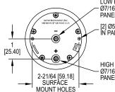
LOW PRESSURE PORT Ø7/16 [11.11] HOLE IN PANEL FOR SURFACE MOUNT
