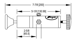
The **Model A-396A Calibration Pump** serves as pressure source to calibrate gages and transmitters or to set pressure switches. Use with manometer or other pressure standard. Includes volume adjuster enabling fine pressure control and bleed valve. Generates pressures from a fraction of an in w.c. to 72 psig (5 bar). Includes barbed fitting, tee connector and three 36" lengths of vinyl tubing.
