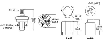
Series A6 Durable Pressure Switches have been specifically designed to stand up to extended duty applications. These switches are constructed with a polyimide film diaphragm and are compatible with a variety of fluids. For ease of installation, the switches come with a 1/4" male NPT process connection and can be mounted in any orientation. The Series A6 pressure switches are compact and have great set point integrity, and feature simple, easy set point field adjustment.
