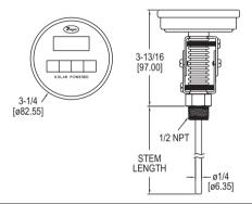
The **SERIES DBT** Digital Solar-Powered Bimetal Thermometer takes the guesswork out of temperature measurement.
