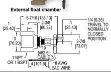
The Series L10 Flotect® Mini-Size Float Switch is a series of economical, compact liquid level floats. It is offered in brass or 303 SS bodies and external tees as well as polypropylene or 304 SS floats with 1" NPT male threads, for direct side mounting through a half coupling, or with factory installed tee for external mounting. This series can be used in liquids with specific gravities as low as 0.5.
