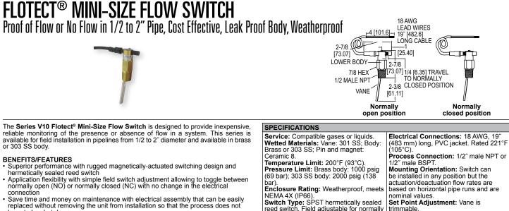
have to be shut down Solves application needs with full size, field-trimmable stainless steel vane provided with removable template calibrated for brass or ductile iron reducing tees with forged steel straight tee/bushing combinations
